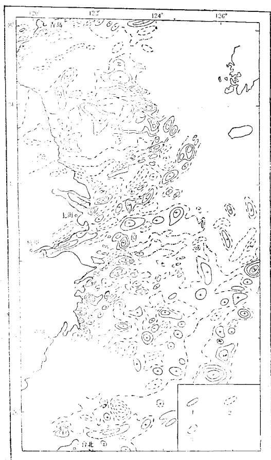
图4 南黄海和东海航磁 \Delta T_a 等值线图 Fig. 4 Schematic isogram of \Delta T_a of airborne magnetic Survey in the region of South Yellow Sea and East China Sea 1.正常值; 2.负异常; 3.0值
