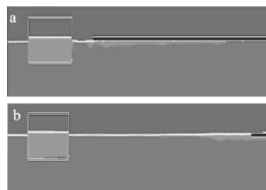
图 5 100 s 时船舶溢油三相物质分布 Fig. 5 Distribution of oil-water-air at 100 s
