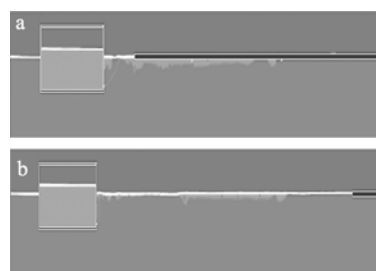
图 4 40 s 时船舶溢油三相物质分布 Fig. 4 Distribution of oil-water-air at 40 s
