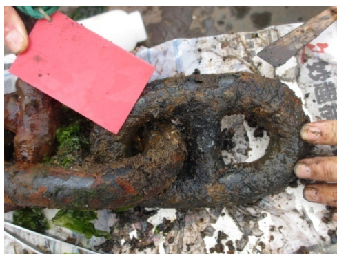
图5 刮除疏松锈层后的底层黑色腐蚀产物 Fig. 5 Black corrosion product obtained after scraping the loose rust layer
