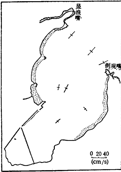
图 1 M_2 分潮流椭圆长短轴分布 (表层) Fig. 1 Distribution of tidal current ellipse axis of M_2 (surface layer) of Xuejiadao Bight in Jiaozhou Bay, Yellow Sea
